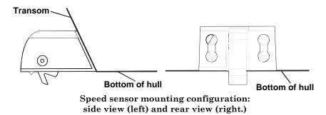
If the base of the transom has a radius, fill the gap between the transom and the sensor with the sealant. This will help ensure a smooth water flow.
